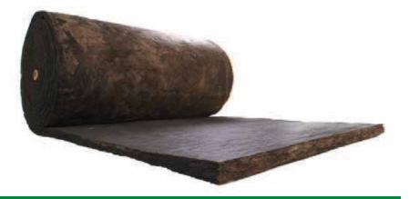
**AKOUSTI-LINER** insulation is a flexible duct liner providing both thermal and acoustical insulation. It is manufactured from inorganic glass fibers bonded with a thermosetting binder. The airstream surface is faced with a black mat bonded to the black fiberglass substrate. AKOUSTI-LINER insulation is offered with or without edge coating to seal fibers.
